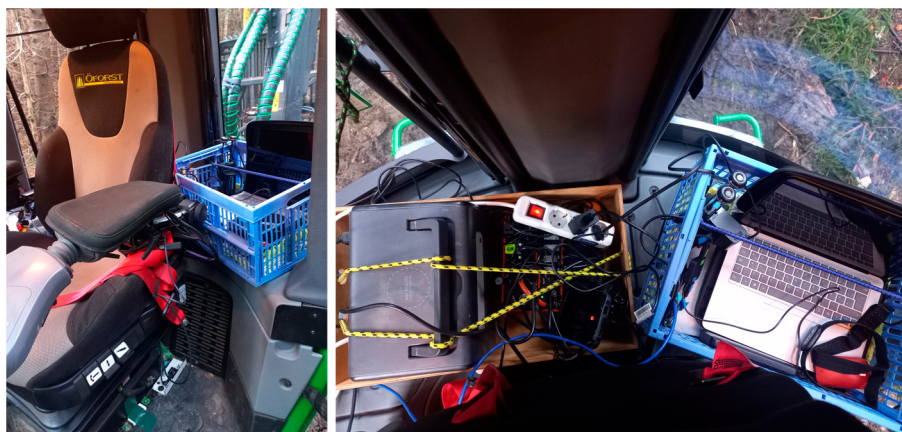
Figure 5. Equipment used to record and synchronize data, which is placed and secured behind the driver's seat.
