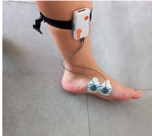
Figure 6. To record EDA data, the sensor is placed on the left foot and the associated electrodes are placed on the instep.
