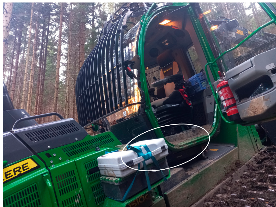
Figure 3. Inclination sensor in a case mounted on the chassis of a forwarder with a tiltable cabin.
