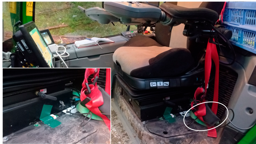
Figure 2. Positioning of the three-dimensional accelerometer and inclination sensors under the driver's seat.
