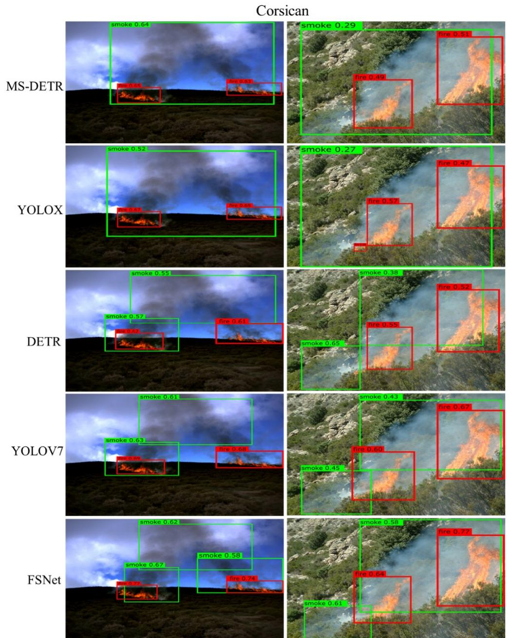
**Figure 6.** The visualized results of smoke recognition by various models on the Corsican dataset. The number in the green detection box indicates the probability of detecting smoke, and the red detection box indicates the probability of detecting fire.
