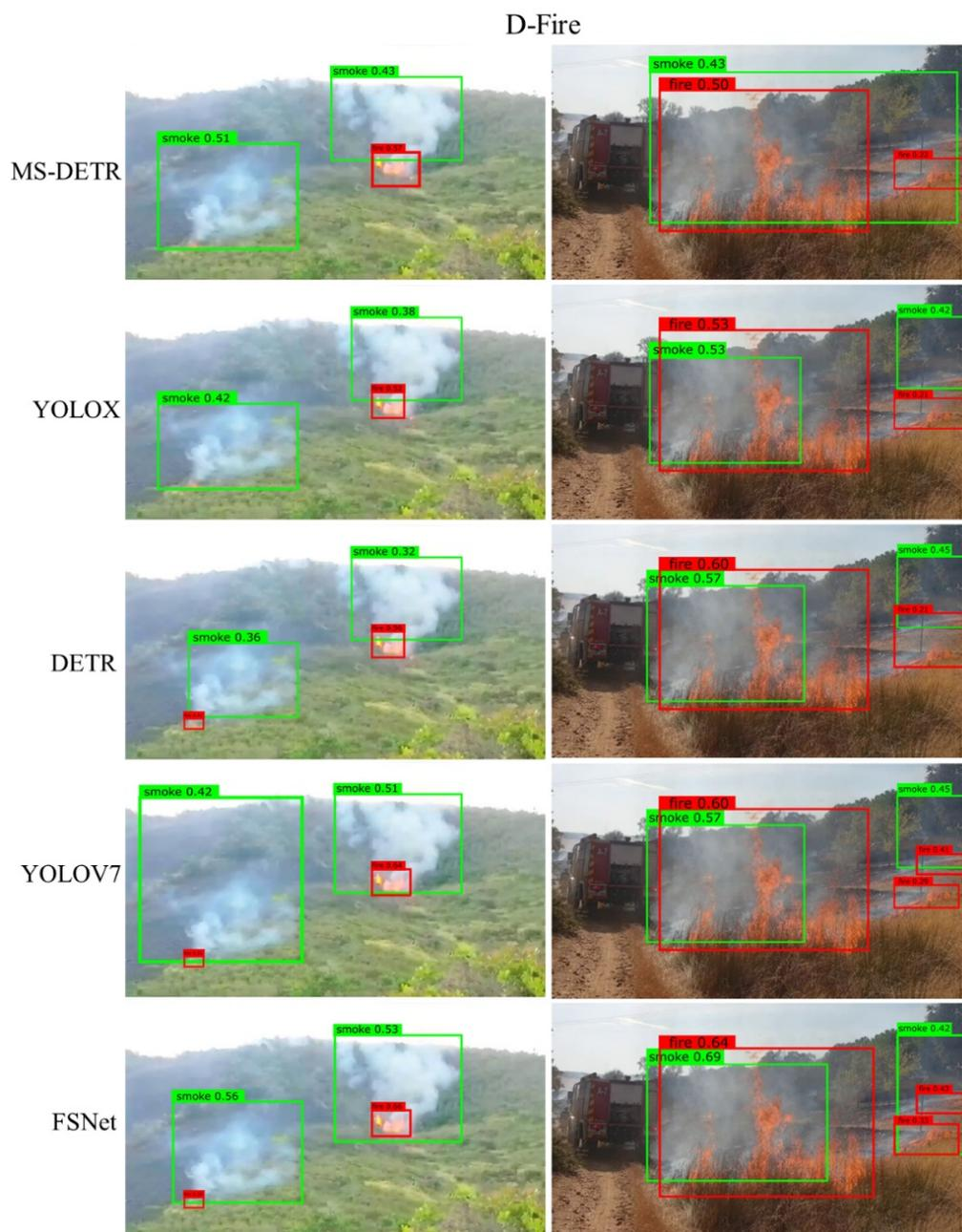
**Figure 7.** The visualized results of smoke recognition using various models on the D-Fire dataset. The number in the green detection box indicates the probability of detecting smoke, and the red detection box indicates the probability of detecting fire.
