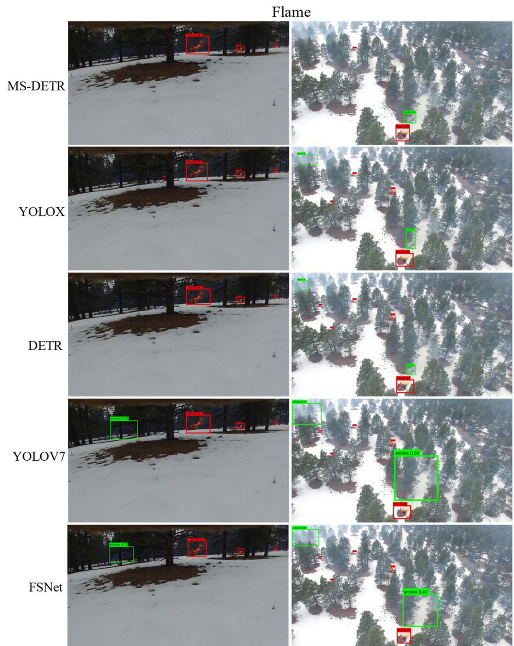
**Figure 5.** The visualized results of smoke recognition by various models on the Flame dataset. The number in the green detection box indicates the probability of detecting smoke, and the red detection box indicates the probability of detecting fire.
