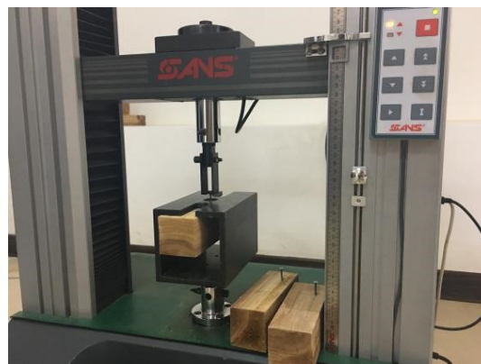
Figure 3. Nail-holding power tests using the mechanical testing machine.
