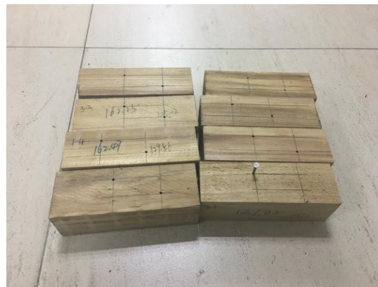
Figure 2. Specimen for nail-holding power.
