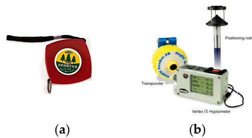
Figure 6. Reference measurement tools for plot data. (a) is the diameter at breast height (DBH) tape; (b) is ultrasonic tree height and range finder (Vertex III).
