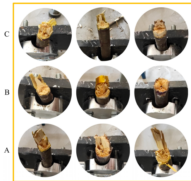
Figure 13. Actual cutting effect. (A) Bionic shark blades; (B) Bionic autocrates aeneus blades; (C) Bionic woodpecker blades.
