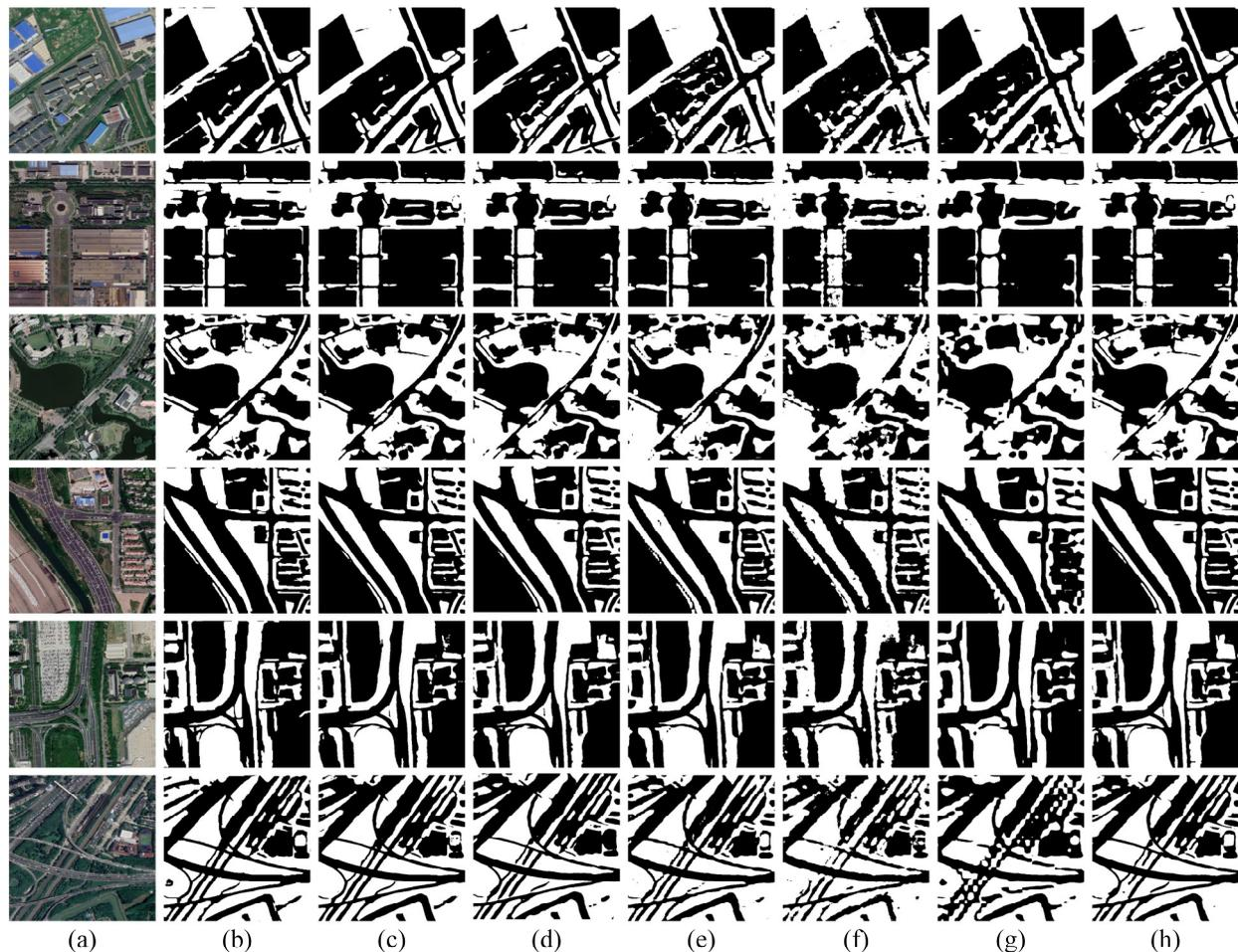
**Figure 11.** UGS segment results using the GS2018 test dataset. (a) Satellite imagery, (b) ground truth, (c) GSRPnet, (d) Unet, (e) PSPnet, (f) Segnet, (g) DeepLab V3+, and (h) SGCNnet.
