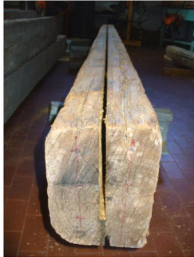
**Figure 2.** Beam no. 3 after the third groove to 75% of the depth.
