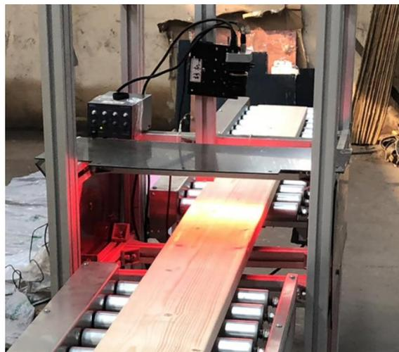
**Figure 14.** Sawn timber inspection equipment based on machine vision technology.
