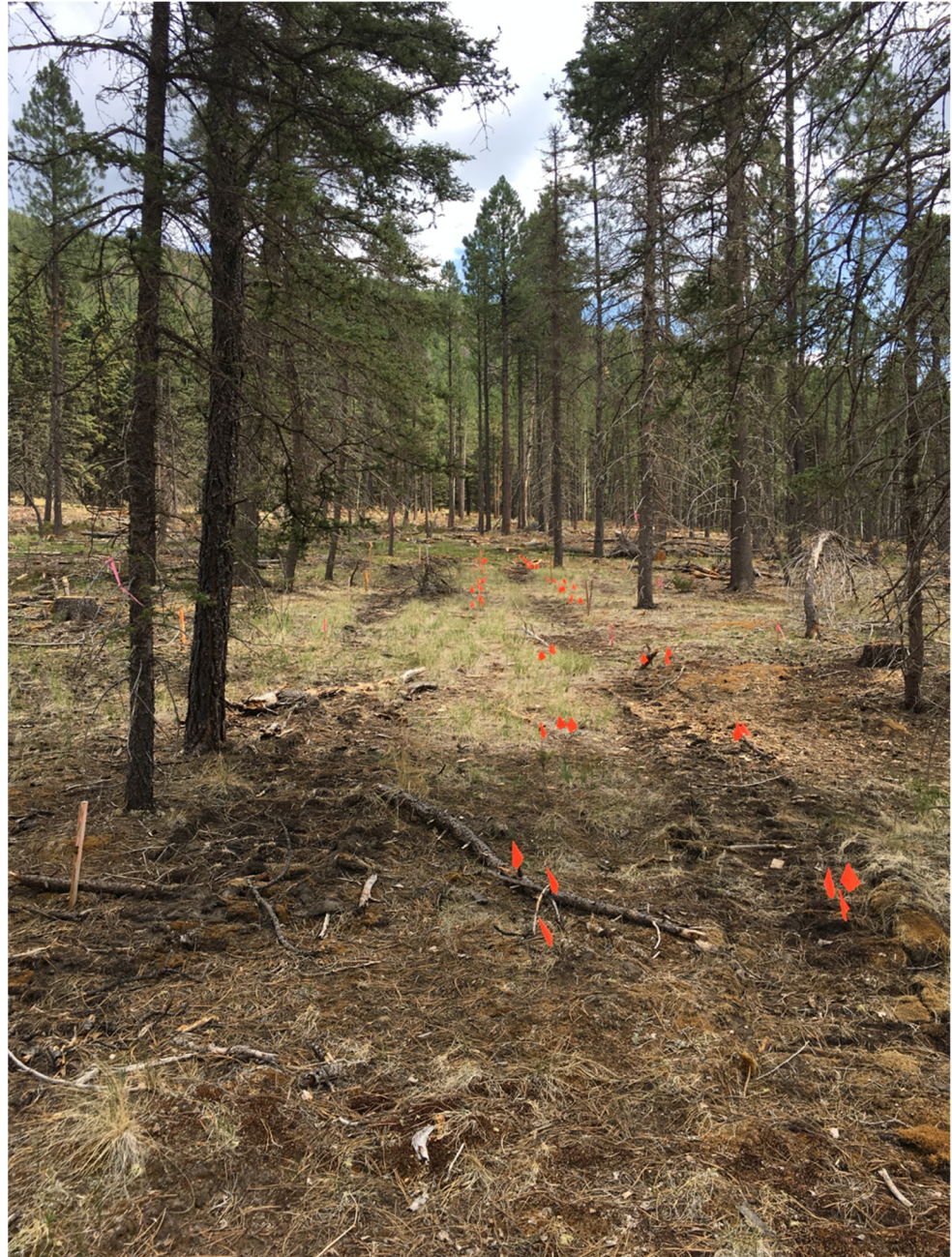
Figure 2. One of three experimental feller buncher disturbance transects. Flags represent sampling points within and between the tracks (each cluster of three flags represents one sampling location). Each of the three transect blocks included three sections treated with 1, 3, and 9 passes, respectively. Samples and measurements were taken at three points per track and intertrack transect section ( N = 54 sampling locations).
