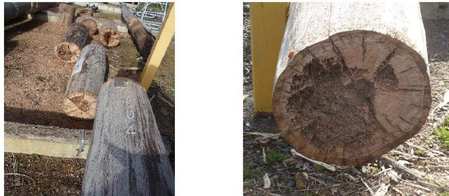
**Figure 3.** Defects in uprooted and sectioned timber poles condemned from service.
