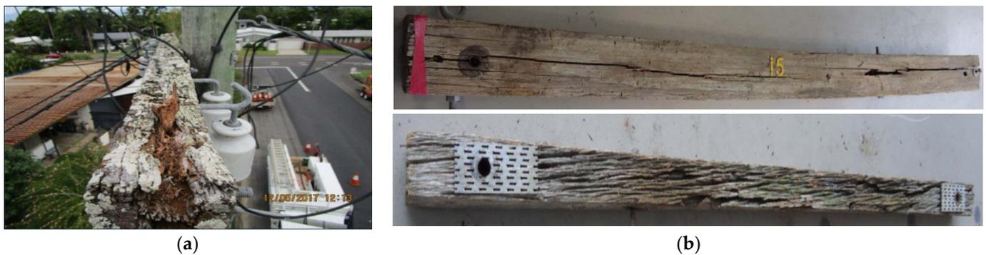
**Figure 4.** Defects in timber cross arms (a) in-service cross arm (b) splitting and weathering in decommissioned cross arms.
