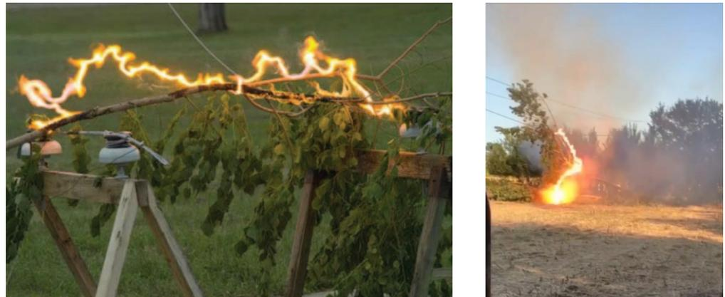
**Figure 2.** Vegetation-related faults and flashover in conductors [20].
