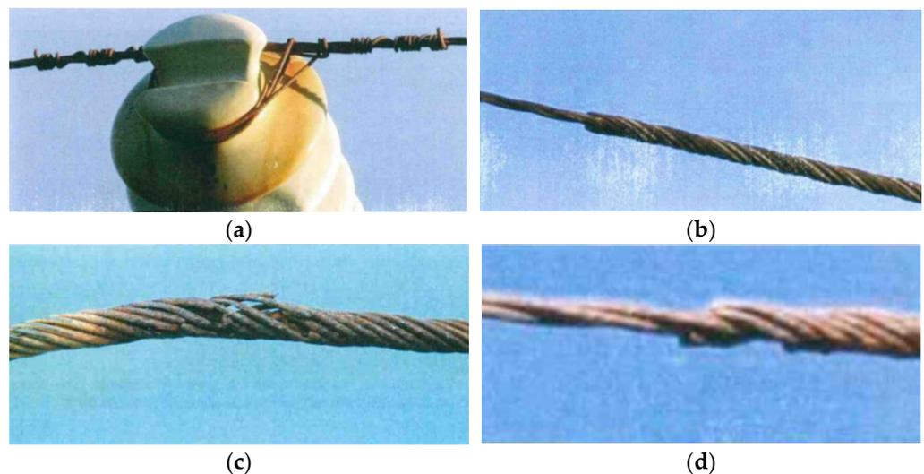
**Figure 6.** Defects in overhead lines. (a) ties (b) terminations (c,d) conductor joints/splices.
