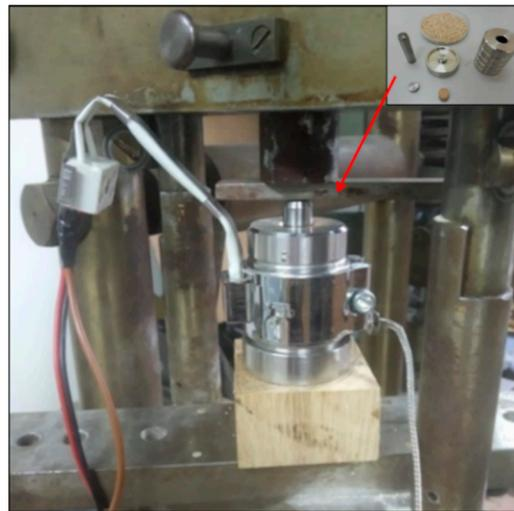
**Figure 1.** Single die press fitted to a Universal Testing Machine.
