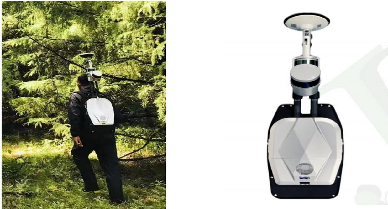
**Figure 3.** LiBackpack DGC50 LiDAR scanning system.
