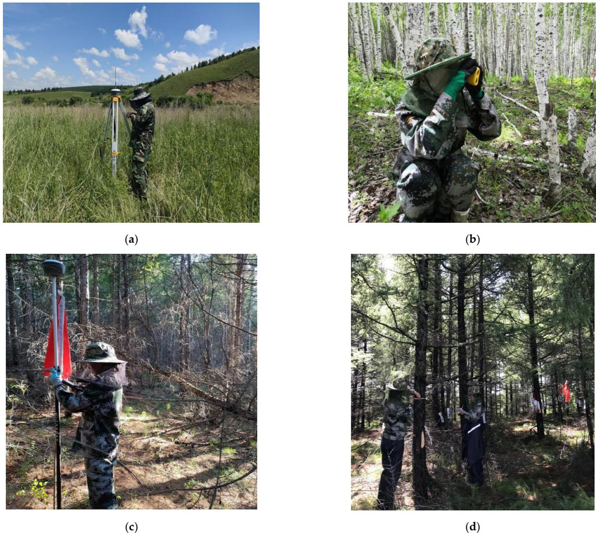
**Figure 2.** (a) Set up base stations. (b) Tree height measurement. (c) Obtain the coordinates. (d) DBH measurement and record.
