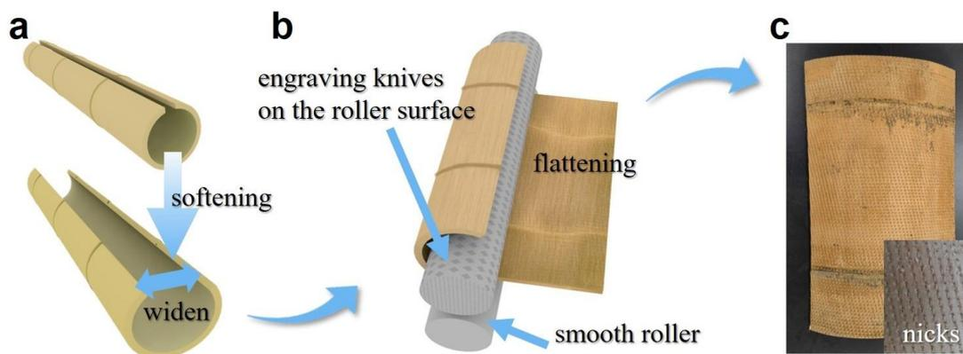
**Figure 2.** Schematic diagrams of (a) bamboo softening and (b) flattening; (c) the physical picture of the FBB inner surface and the enlarged view in the lower-right corner.
