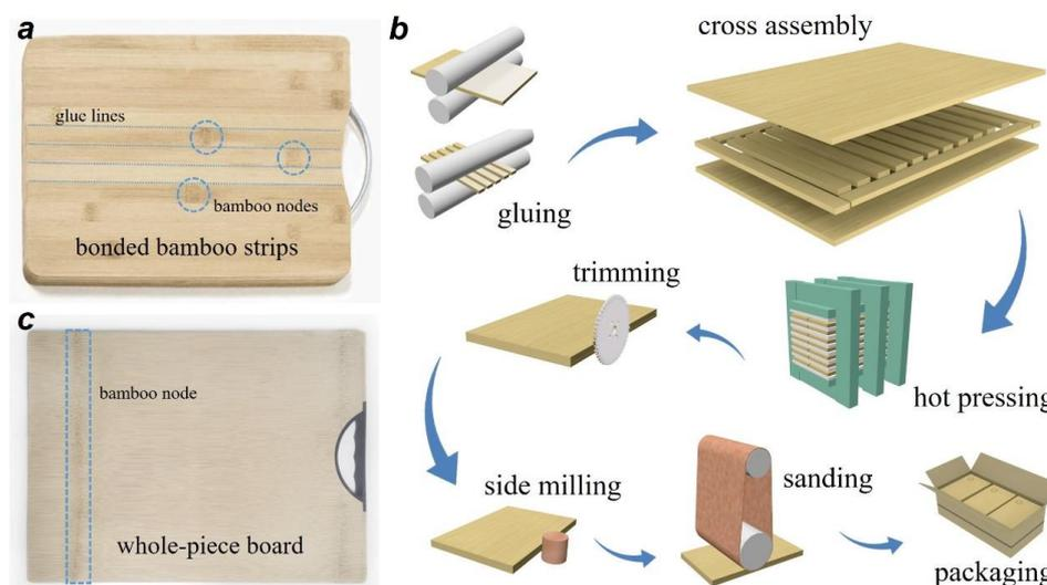
**Figure 6.** (a) Presentative picture of the laminated bamboo chopping board; (b) schematic of the production process of FBCB; (c) presentative picture of FBCB.
