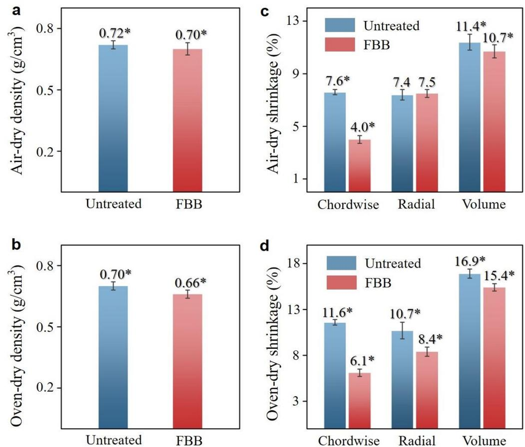
**Figure 4.** Comparison of (a) air-dry density, (b) oven-dry density, (c) air-dry shrinkage and (d) oven-dry shrinkage of bamboo before and after flattening modification. The data in the graph are average values and the error bars represent standard deviations. Values followed by “\*” indicate that the *p*-value of the *t*-test is less than 0.05, and significant differences appear between untreated and FBB data, while unmarked values indicate no significant differences.
