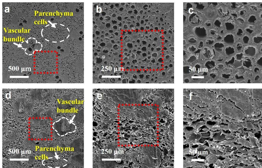
**Figure 3.** SEM images of (a–c) untreated bamboo and (d–f) FBB.
