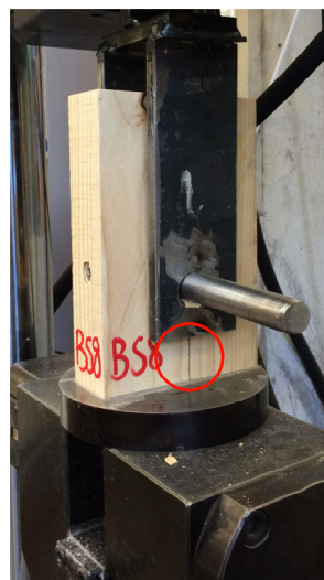
Figure 6. Camera captured the crack propagation on the surface of a reinforced specimen.
