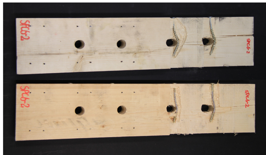
Figure 11. Timber members of connection specimens after failure showing deformation of screws. Top: connections reinforced by screws with complete thread (SFC). Bottom: connections reinforced by screws with 33% thread on the point end (SPC) [31].
