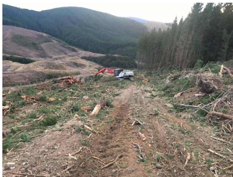
Figure 5. Skid trail A in operation, leading down to the shovel. The deep disturbance measure was almost exclusively from the main skid trails.
