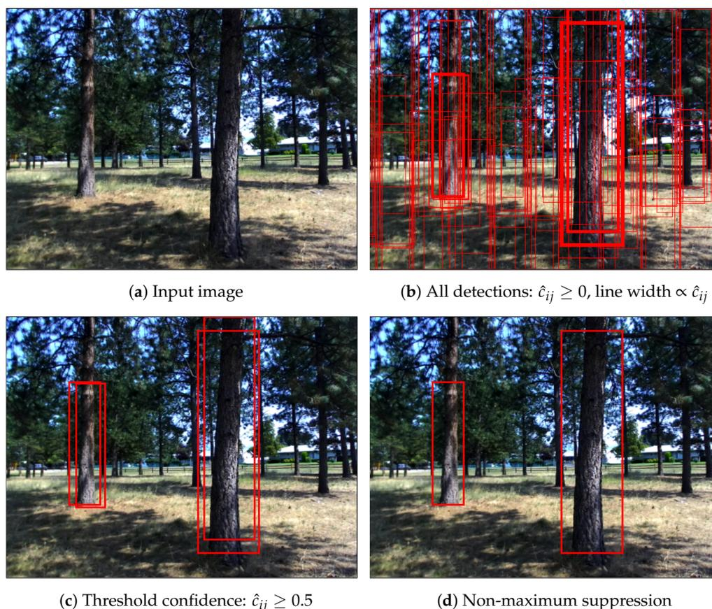
**Figure 2.** Inference pipeline: (a) Input image. (b) All predictions after forward pass through the network. Line widths are proportional to confidence. (c) Retained predictions after thresholding on the confidence. (d) Final prediction following non-maximum suppression.
