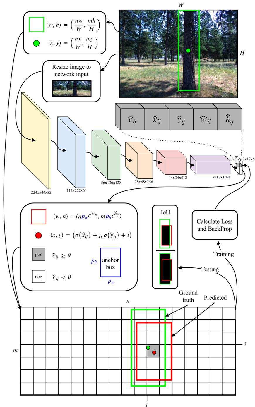
Figure 1. Conceptual diagram of the detection algorithm.
