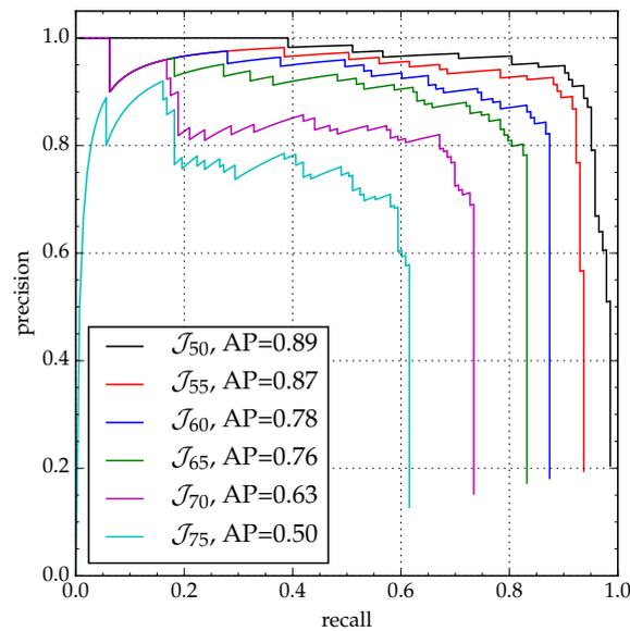
**Figure 4.** Precision–recall curves for the tree stem detection algorithm.
