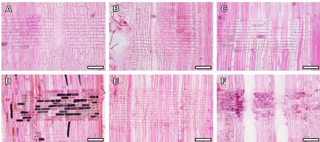
**Figure 7.** Optical micrographs of the radial sections of (A) *Q. variabilis*, (B) *Q. serrata*, (C) *Q. mongolica*, (D) *Q. dentata*, (E) *Q. aliena*, and (F) *Q. acutissima*. Scale bar: 100  $\mu$ m.
