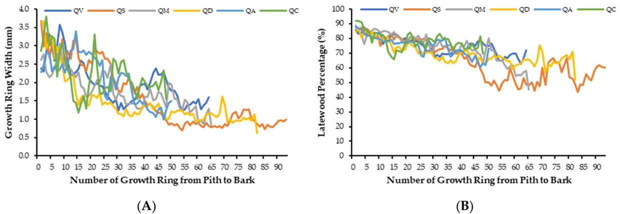
**Figure 5.** Radial variation in (A) growth ring width and (B) latewood percentage of *Q. variabilis* (QV), *Q. serrata* (QS), *Q. mongolica* (QM), *Q. dentata* (QD), *Q. aliena* (QA), and *Q. acutissima* (QC). The results are the averages of three trees.
