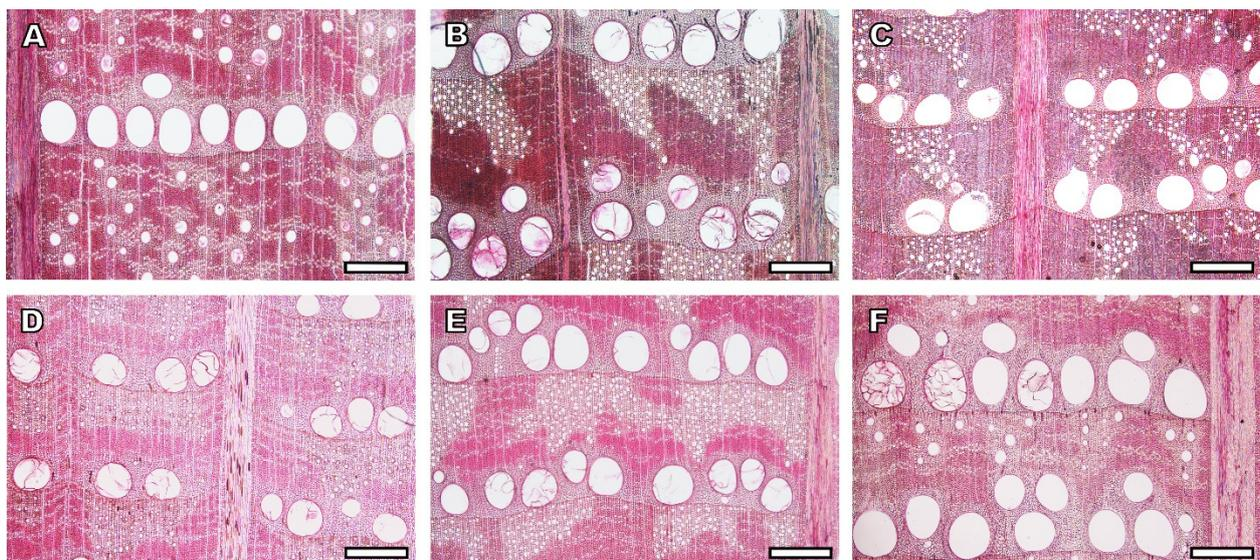
**Figure 6.** Optical micrographs of the cross-sections of (A) *Q. variabilis*, (B) *Q. serrata*, (C) *Q. mongolica*, (D) *Q. dentata*, (E) *Q. aliena*, and (F) *Q. acutissima*. Scale bar: 500  $\mu$ m.
