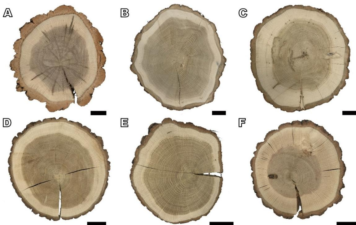
**Figure 2.** Wood disks of (A) *Q. variabilis*, (B) *Q. serrata*, (C) *Q. mongolica*, (D) *Q. dentata*, (E) *Q. aliena*, and (F) *Q. acutissima*. Scale bar: 5 cm.
