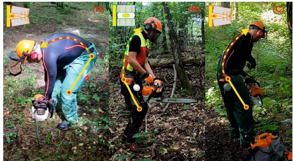
Figure 3. Visual display of workers’ spine flexion regarding three methods of starting a chainsaw (A) from the ground, (B) between the knees, (C) “drop starting”.
