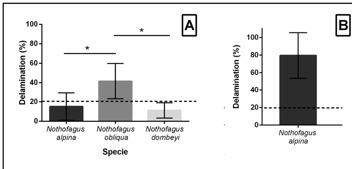
**Figure 5.** Summary of delamination test value. (A) Results using dry and (B) native timber conditioned. The asterisk indicates a significant difference ( $p < 0.05$ ). The dashed line indicates the standard value required.
