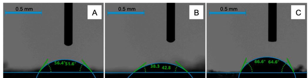
**Figure 8.** Image of a drop of water in contact with the surface of the wood before gluing with naturally dried timber at a temperature of 20 °C, with a detection time of 3 s for (A) *Nothofagus alpina*, (B) *Nothofagus obliqua*, and (C) *Nothofagus dombeyi*.
