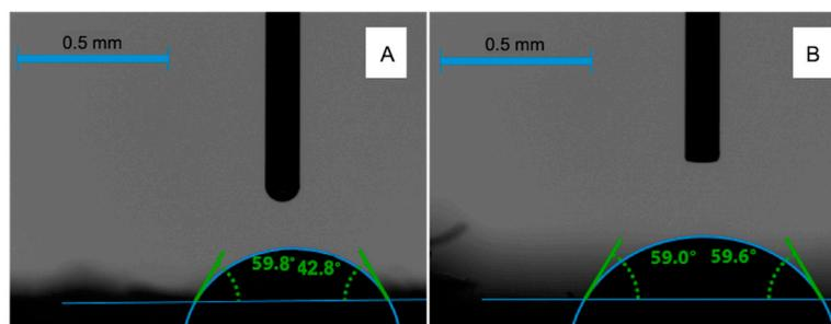
**Figure 9.** Image of a drop of water in contact with the wood surface before gluing with naturally moist timber at a temperature of  $20^\circ\text{C}$ , with a detection time of 3 s for (A) *Nothofagus alpina* and (B) *Nothofagus obliqua*.
