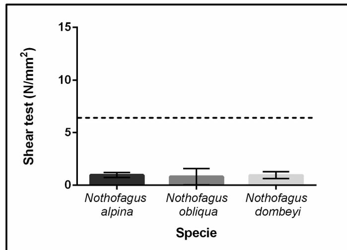
**Figure 4.** Shear test values using moisture timber of native species. The dashed line indicates the standard value required.
