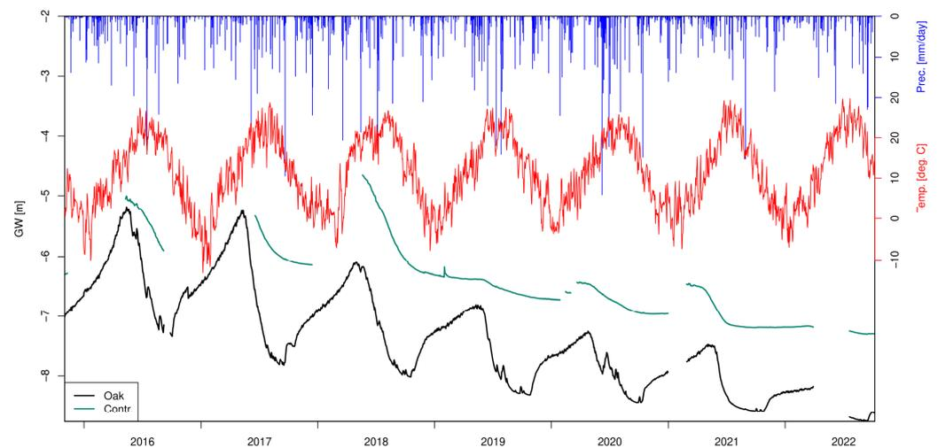
**Figure 5.** Daily precipitation, air temperature, and groundwater levels in the forest and control monitoring sites between 2016 and 2022. Blue columns—precipitation; red line—temperature; green line—groundwater level at the control point; black line—groundwater level at the forested point.
