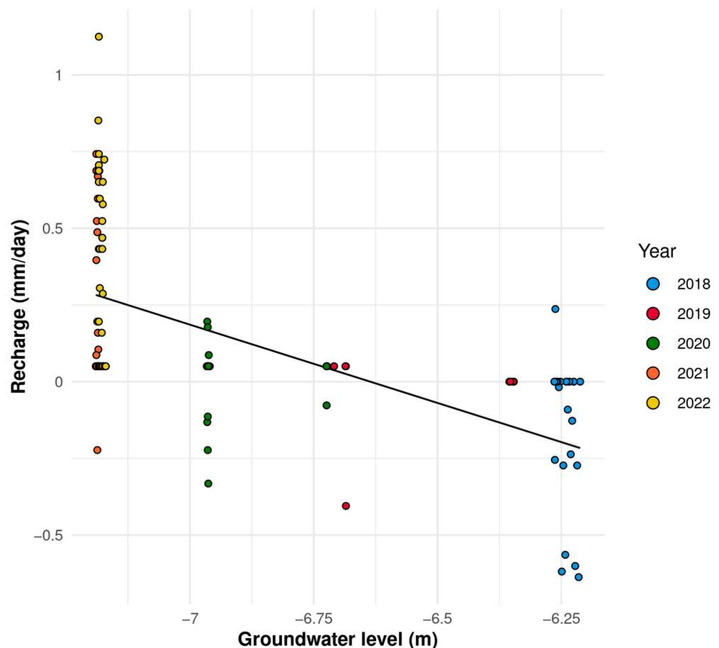
**Figure 8.** Relationship between the recharge and groundwater level during the dormant period under the control point ( $R^2 = 0.332$ ).
