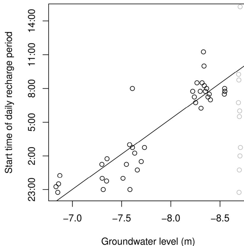
**Figure 12.** Relationship between the start of the daily recharge periods and groundwater level during the vegetation period under the forest sample point. The data from 2022 are in light grey ( $R^2 = 0.810$ ).
