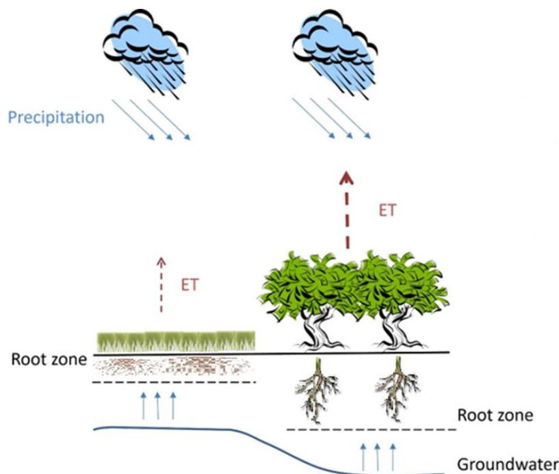
**Figure 1.** Schematic representation of the differences in water uptake between forests and herbaceous vegetation. ET: evapotranspiration.
