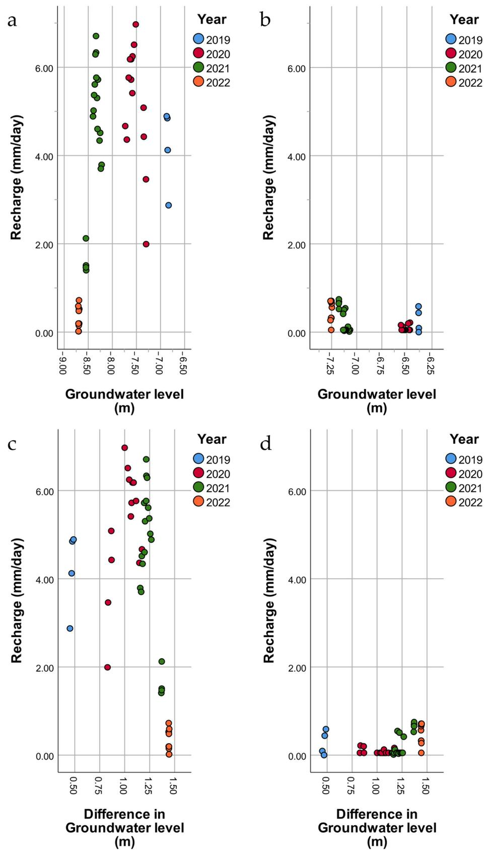
Figure 9. Relationship between the groundwater level recharge and groundwater level (a: Oak; b: Control) and difference in groundwater levels (magnitude of the depression) between the control and forest wells (c: Oak; d: Control) during the vegetation period.
