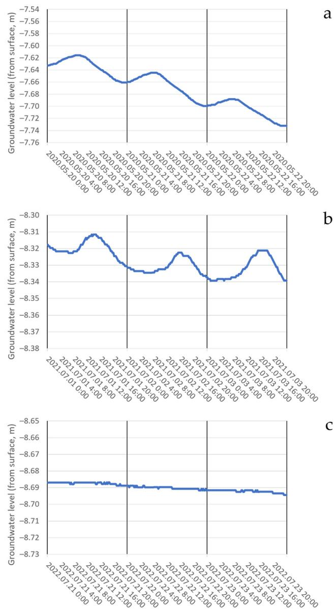
**Figure 11.** (a–c) Daily groundwater level fluctuations under the forest in 2020 (a), 2021 (b), and 2022 (c) on three consecutive precipitation-free days. The vertical lines indicate midnight on each day.
