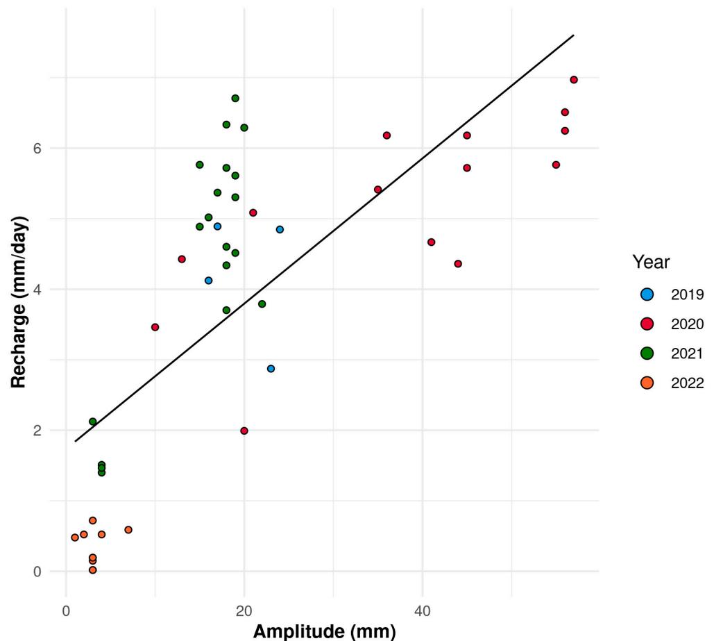
**Figure 10.** Relationship between the groundwater level recharge and amplitude of the daily groundwater fluctuations during the vegetation period under the forest sample point ( $R^2 = 0.548$ ).
