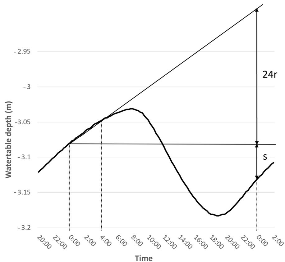
**Figure 3.** Schematic representation of the White method (based on Gribovszki [63]).
