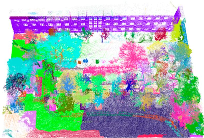
**Figure 7.** DMS dataset hyper-segmentation effect. Different adjacent colors represent different semantic blocks, and blocks with similar semantic information are allocated to the same block. For example, purple represents buildings with high semantic consistency, while individual trees are divided into multiple areas.
