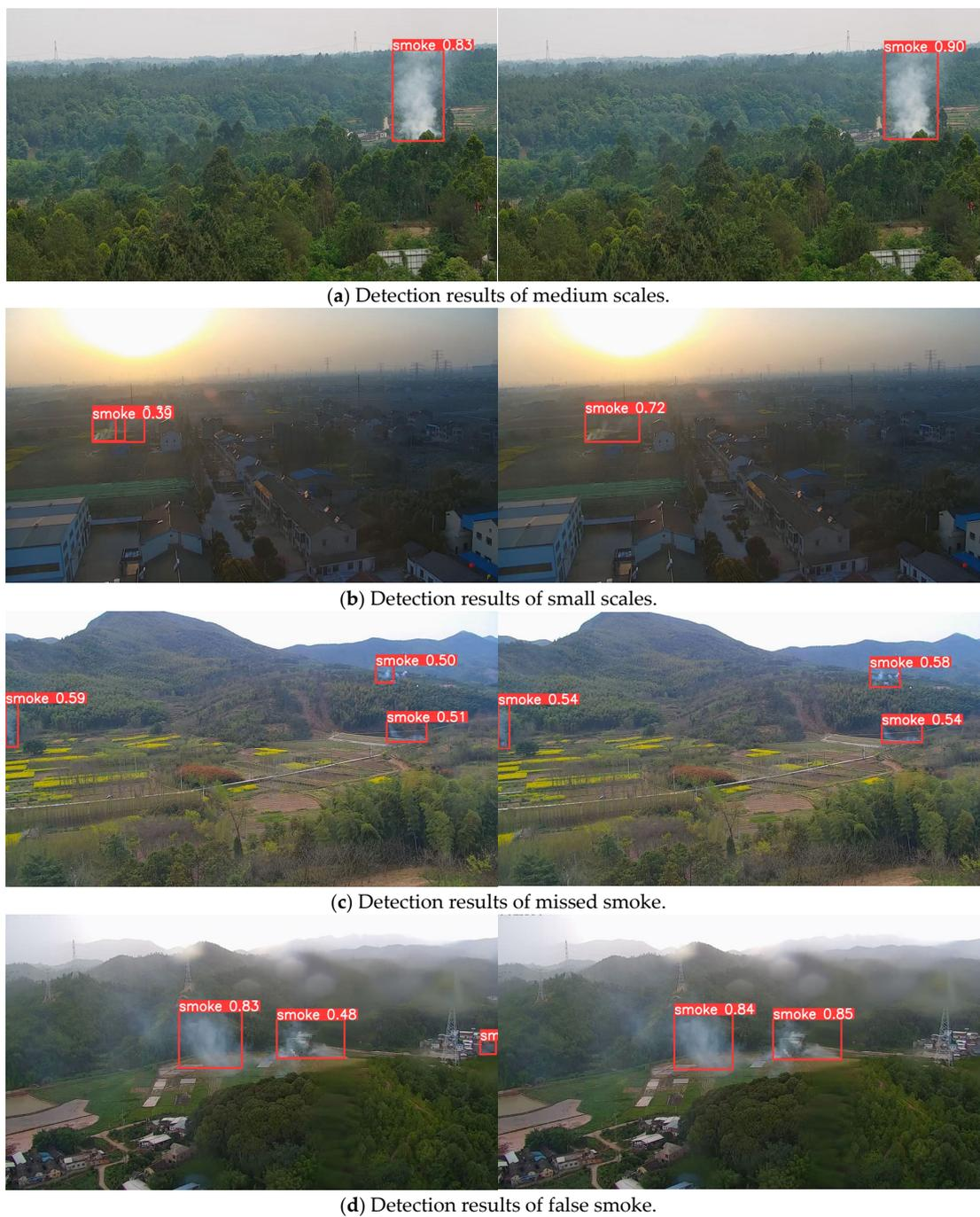
**Figure 7.** Detection effect before (left) and after (right) the improvement: (a,b) smoke at different percentage detection results; (c,d) missed and false detection results.
