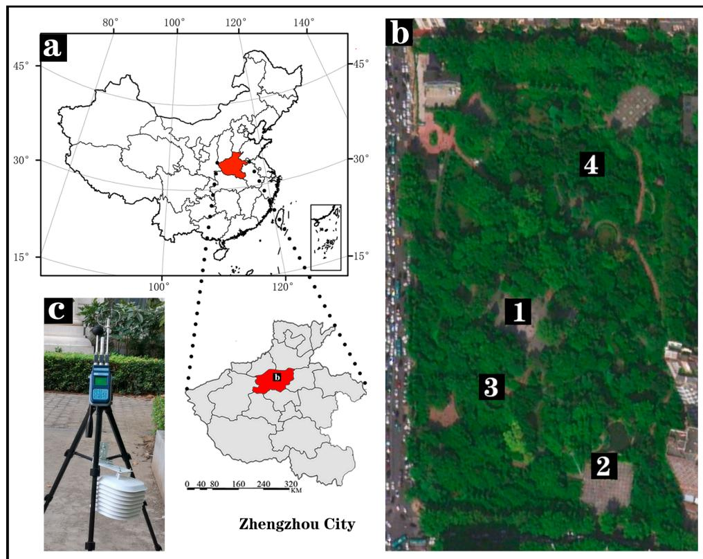
**Figure 1.** (a) Location of Zhengzhou; (b) Google Earth map of the study area, Lvyin Park and sample points include unshaded location (1) and (2), tree-shaded location (3) and (4); (c) measurement instruments.
