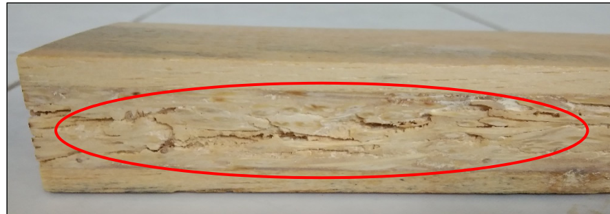
Figure 5. Failure of laminated compreg composites pressed with 30% CR.
