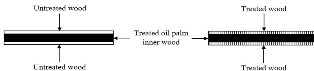
Figure 1. Product description for laminated *compreg* composite products.
