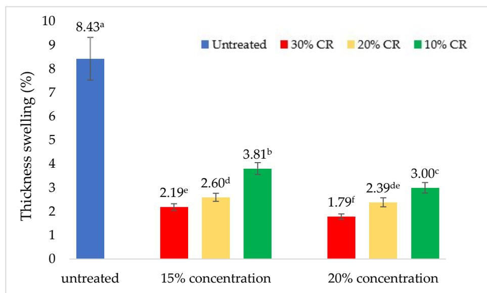
**Figure 2.** Thickness swelling of compreg oil palm inner wood.
