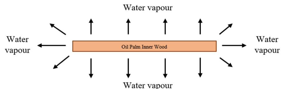
**Figure 6.** Water vapor is released from a sample of compreg oil palm inner wood during compression.
