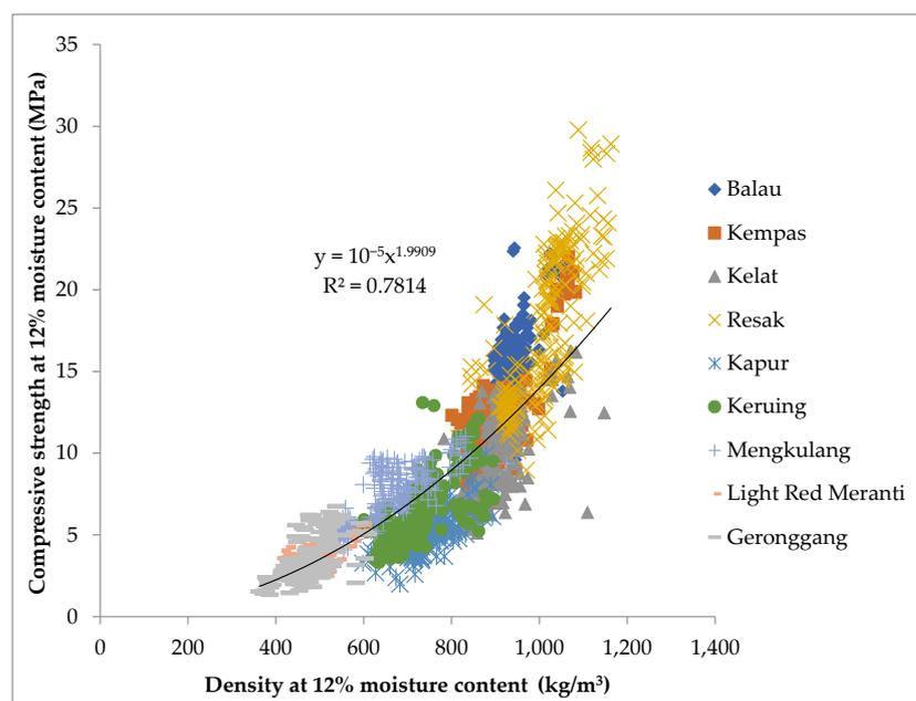
**Figure 7.** Relationship between compressive strength perpendicular to the grain and density for selected Malaysian tropical hardwood timbers.
