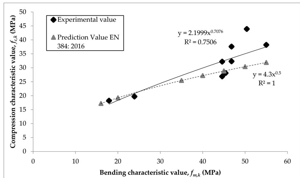
**Figure 8.** Relationship between experimental and derivative compressive and bending strength characteristic values.
