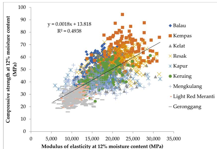
**Figure 4.** Relationship between compressive strength parallel to the grain and modulus of elasticity for selected Malaysian tropical hardwood timber.
