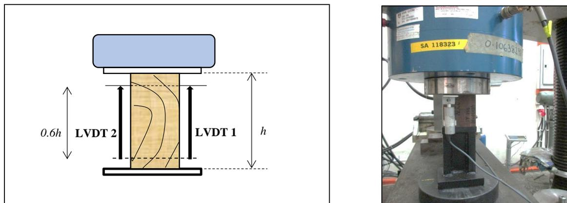
**Figure 3.** Test setup for determining compressive strength properties perpendicular to the grain.
