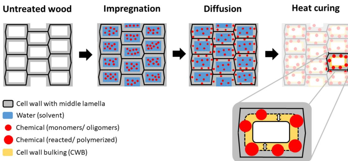
**Figure 7.** Schematic illustration showing the effects of chemical wood modification on cellular level from impregnation with a chemical diluted in a solvent (e.g., water) to drying and curing of the monomeric modification reagent causing a cell wall bulking (CWB).
