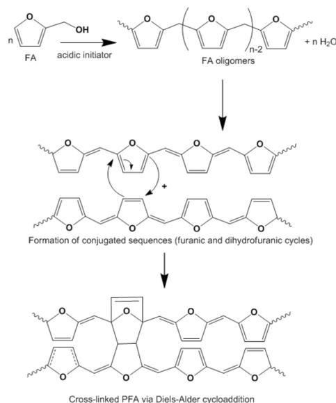
**Figure 2.** Schematic for polymerization of furfuryl alcohol.
