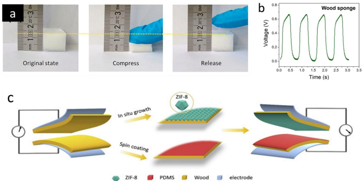
**Figure 10.** (a) Compressibility of wood sponges obtained by delignification of balsa wood and (b) the corresponding piezoelectrical output. Reprinted with permission from [325]. Copyright 2020 American Chemical Society. (c) Functionalization of a wood-based triboelectric nano-generator [327].
