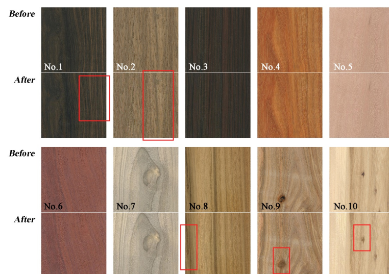
Figure 1. Ten hardwood grain images before and after the Gaussian histogram specification.
