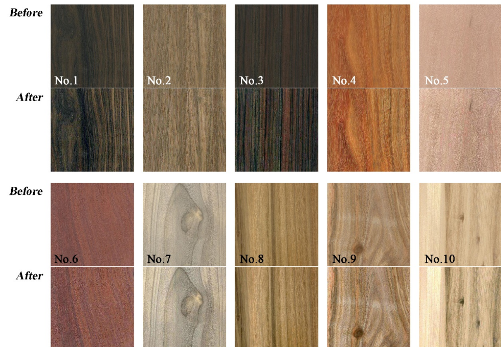
Figure 5. Ten Gaussian hardwood grain images before and after the adaptive color adjustment.
