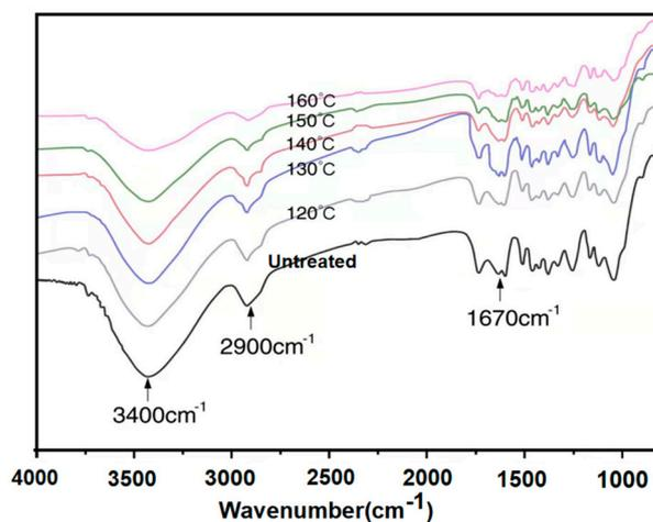
Figure 2. FTIR spectra for bamboo samples.
