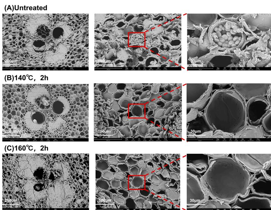
**Figure 5.** SEM images of bamboo samples hydrothermally treated at different temperatures for 2 h.
