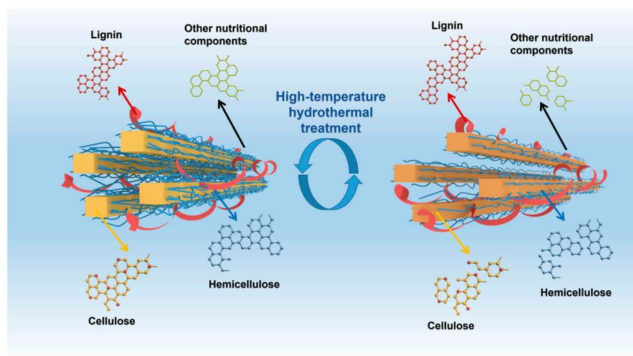
**Figure 4.** Schematic diagram of chemical composition changes of moso bamboo under high-temperature hydrothermal treatment.
