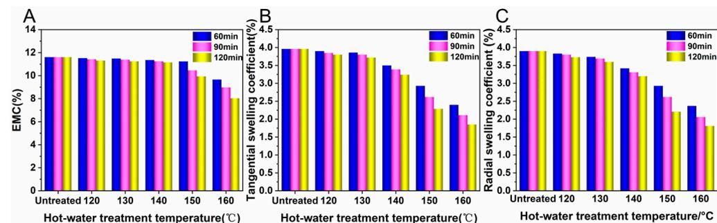
**Figure 7.** (A) Influence of different hydrothermal treatments on EMC; (B) Influence of different hydrothermal treatments on tangential swelling coefficient; (C) Influence of different hydrothermal treatments on radial swelling coefficient.
