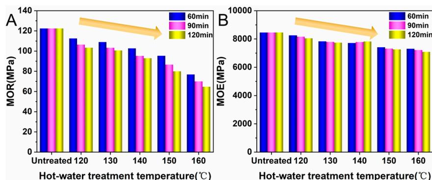
**Figure 6.** (A) Influence of different hydrothermal treatments on MOR of samples; (B) Influence of different hydrothermal treatments on MOE of samples.
