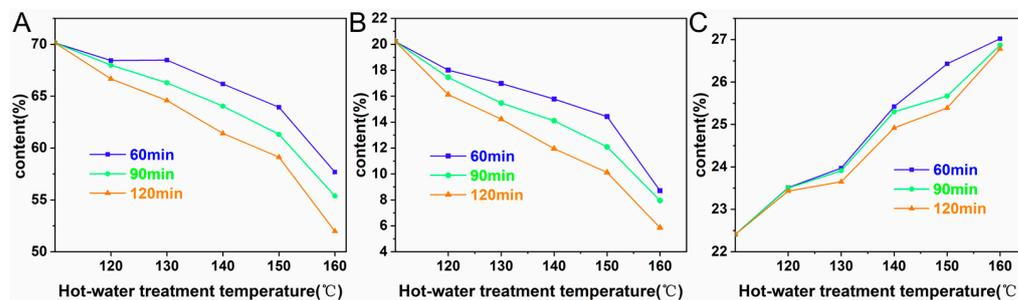
**Figure 3.** Influence of hydrothermal treatments on the main chemical composition of bamboo samples: (A) Cellulose; (B) Hemicellulose; (C) Lignin.
