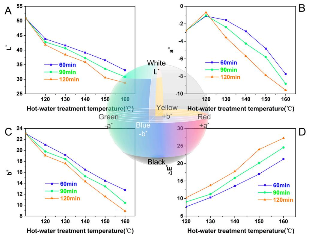
**Figure 8.** (A) Influence of different hydrothermal treatments on  $L^*$ ; (B) Effect of different hydrothermal treatments on  $a^*$ ; (C) Effect of different hydrothermal treatments on  $b^*$ ; (D) Effect of different hydrothermal treatment on  $\Delta E^*$ .
