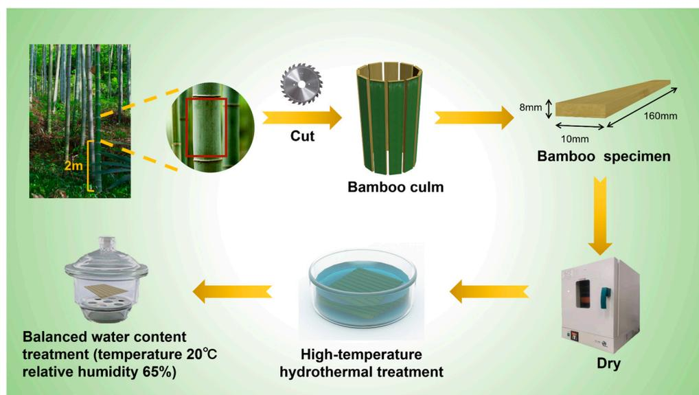
**Figure 1.** The high-temperature hydrothermal treatment process of moso bamboo specimens.
