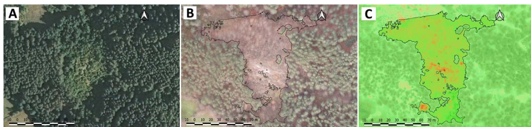
Figure 3. GIS application for determination of the boundaries of bark beetle spots in Kremen region: (A) aerial 2011 RGB image; (B) UAV 2019 RGB image; (C) UAV 2019 NDVI image.
