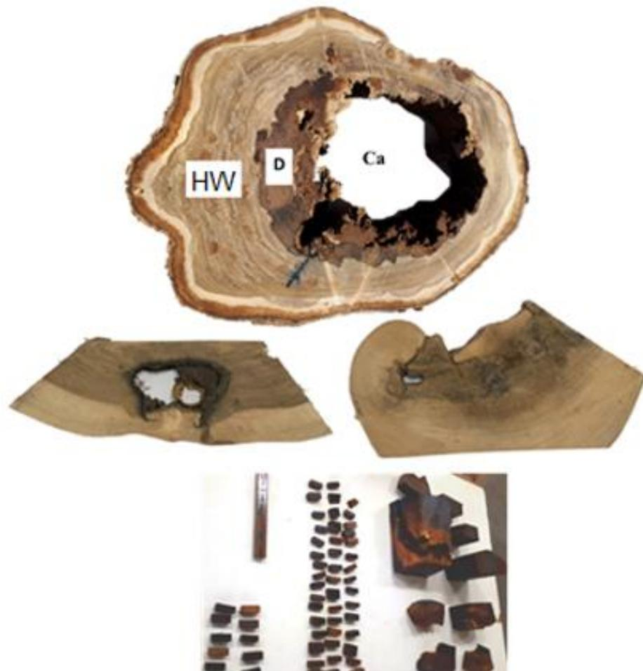
**Figure 4.** Upper image: Cross-sections after polishing showing demarcation of the healthy wood regions (HW), deteriorated wood (D) and cavity (Ca); Intermediate image: cross-section cuts in different demarcated regions; lower image: specimens taken from different demarcated regions.
