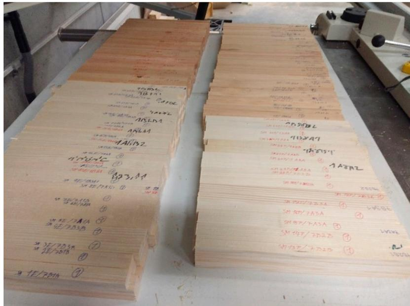
**Figure 2.** Glued wood samples.
