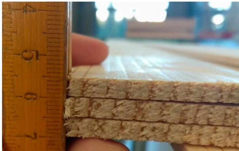
**Figure 1.** Wood lamellae for specimens.
