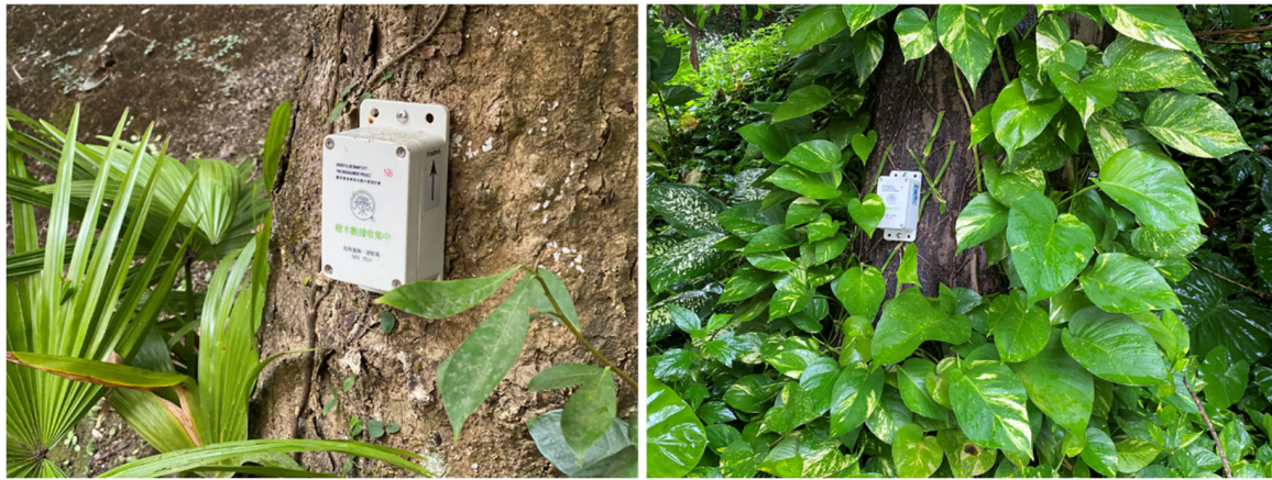
Figure 3. Sensors are fixed with the appropriate length of the screw at the position at the lower tree trunk at the height of 0.5 m or the lowest reachable position near the ground.
