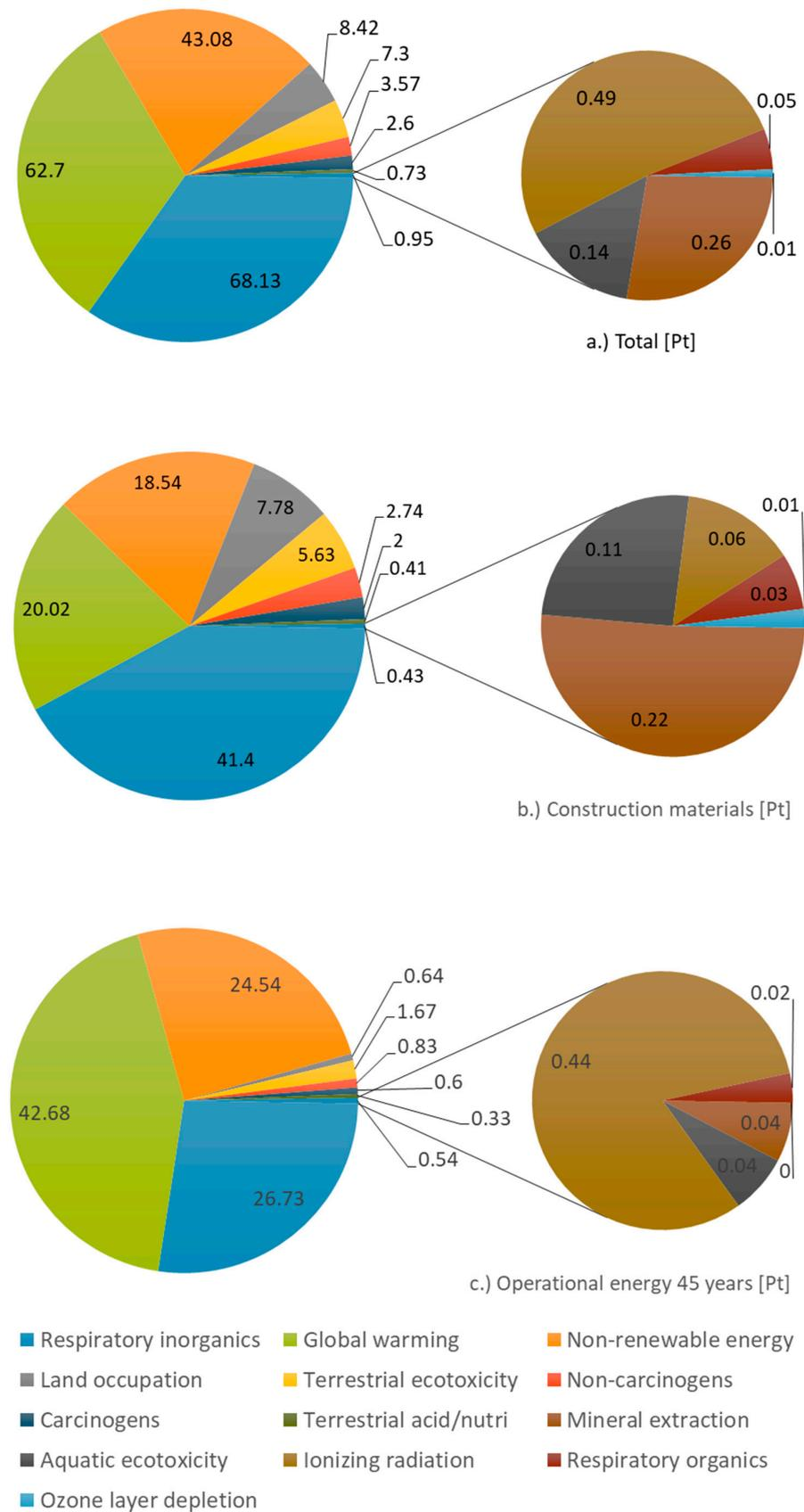
**Figure 3.** Environmental impact comparison of construction materials and operational energy demands for 45 years of the NZEB-W; IMPACT2002+ method; midpoints single score Pt (Eco-indicator point).
