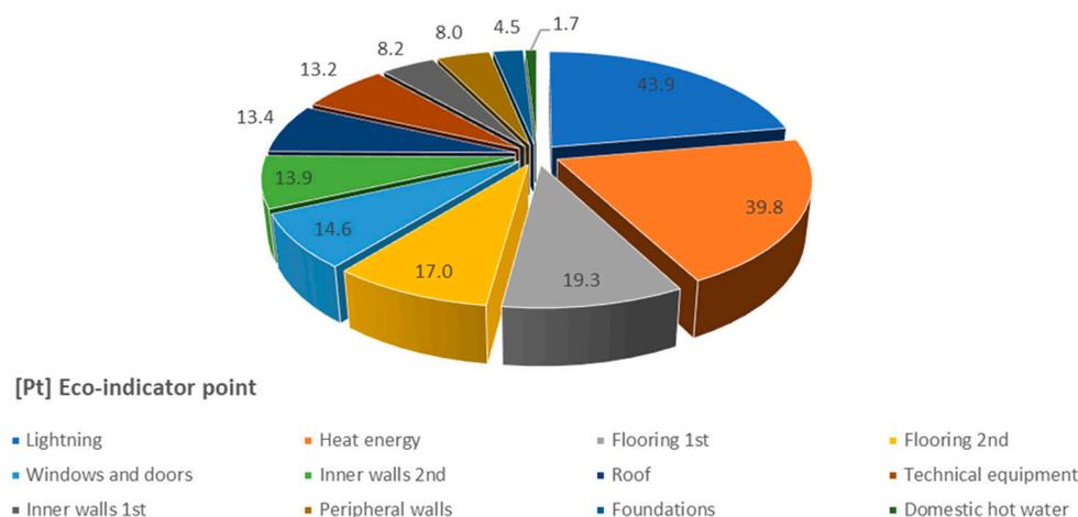
**Figure 4.** Environmental impact comparison of the construction materials and operational energy demands for 45 years (lightning, heat energy, technical equipment, domestic hot water) of the NZEB-W in structural unit; IMPACT2002+ method; single score Pt (Eco-indicator point).
