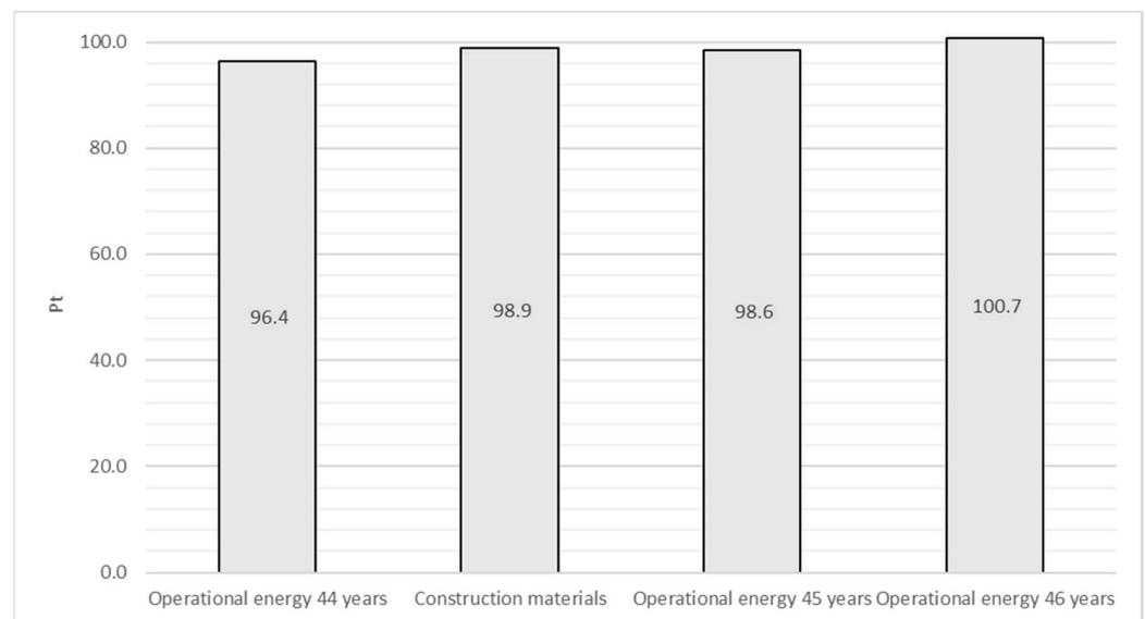
**Figure 2.** Environmental impact comparison of the construction materials and operational energy demands for 44, 45, and 46 years of the NZEB-W; IMPACT2002+ method; single score Pt (Eco-indicator point).
