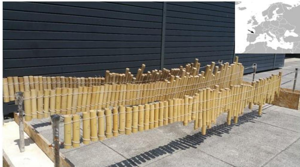
**Figure 1.** The 6 month weather exposure durability test and geographical location of the test (see map in upper right).
