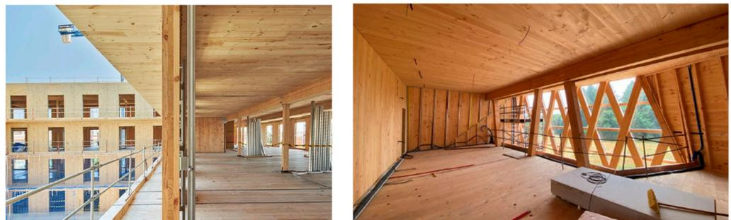
**Figure 1.** Residential building in Cornellá and Green Impulse Building in Lugo, build using GLT and CLT of Radiata pine (Source: Ref. [16]).
