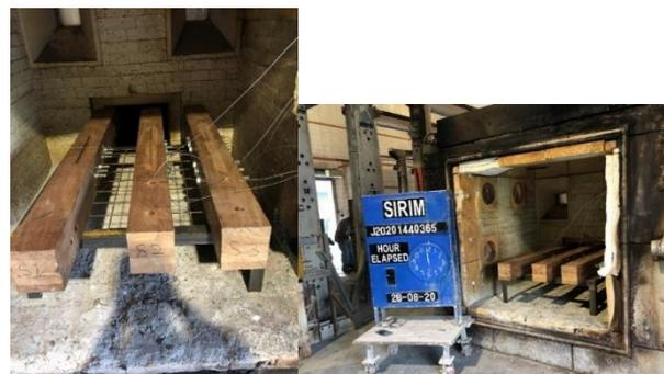
**Figure 5.** Experimental Preparation of the Samples in the Furnace.
