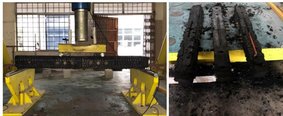
**Figure 7.** Experimental Four-point Bending Test Set-Up After Exposure to Standard Fire.
