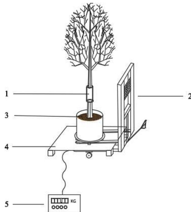
**Figure 1.** Schematic diagram of experimental set-up: (1) thermal dissipation probe, (2) portable forklift, (3) plastic film, (4) wide-range balance, (5) display screen.
