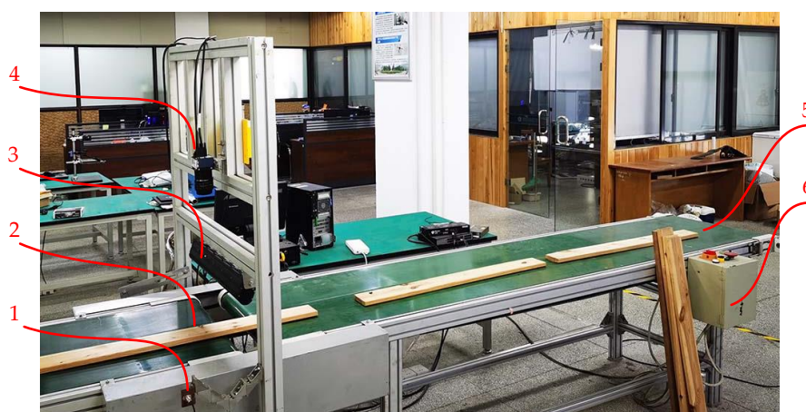
Figure 1. Image acquisition device: (1) photoelectric sensor, (2) solid wood board, (3) linear light source, (4) CCD camera, (5) belt conveyor, and (6) sample solid wood floorboard.
