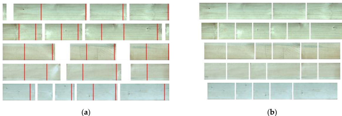
Figure 6. Elite retention genetic algorithm sawing results. (a) Planned cutting points. (b) Wood after sawing.
