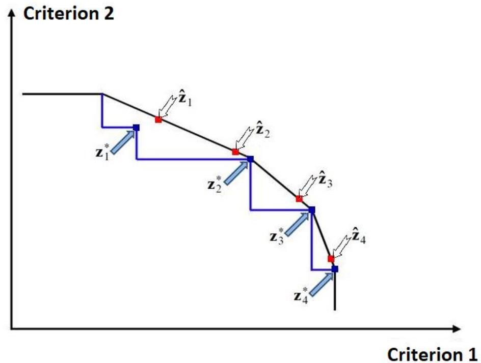
**Figure 3.** Validation scheme. Red dots represent the point selected in the surrogate frontier ( $\hat{z}_s$ ). Blue dots are the feasible solutions ( $z_s^*$ ) for MOIP.
