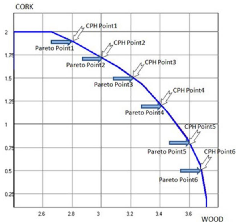
**Figure 6.** Accuracy of the convex Edgeworth–Pareto hull (cEPH) with respect to the Pareto frontier for the Penafiel model. White arrows represent the points in the cEPH and blue arrows the location of the nearest point in the real Pareto frontier.
