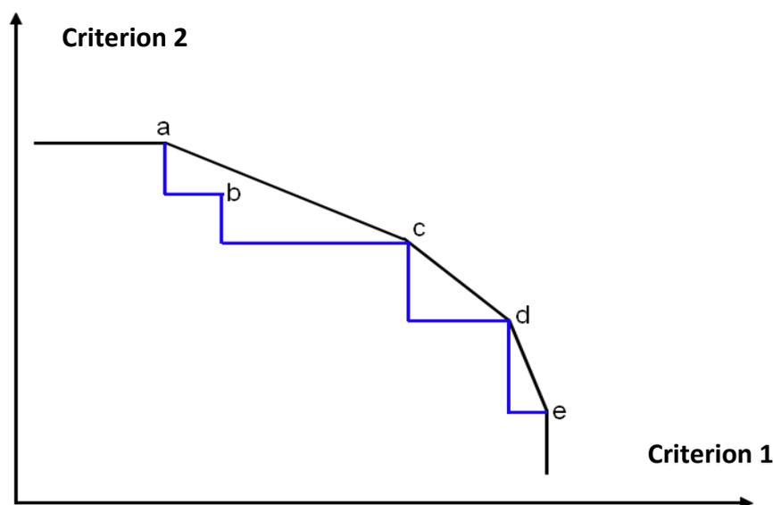
**Figure 2.** Approximation of the Pareto frontier by its convex hull (the surrogate frontier). The blue line represents the Pareto frontier for an integer variable model; the black line—convex Pareto hull for the same model.
