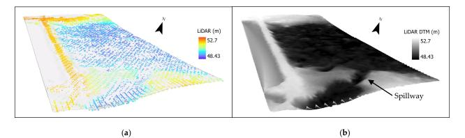
Figure 5. Bare-earth returns from the LiDAR point cloud (a) and the extracted DTM of the study site (b).
