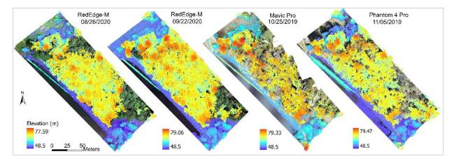
Figure 3. The height-colored point clouds extracted from four flights (RE0826, RE0822, MP1025, and P41106).
