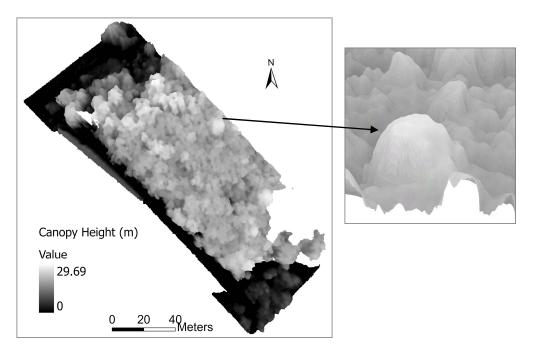
Figure 6. The CHM from the RE0922 mission. The inset shows a 3D view of the example pine tree.
