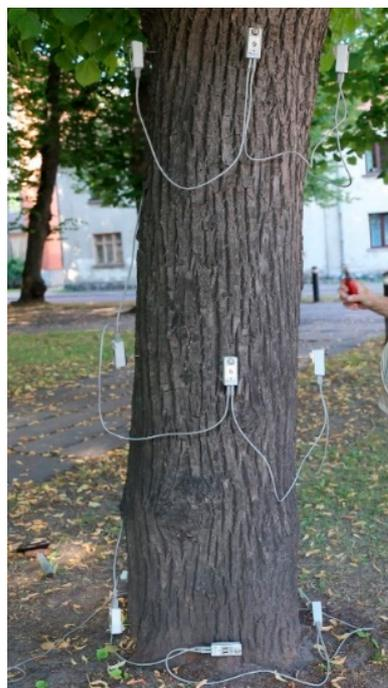
**Figure 3.** The use of acoustic tool ARBOTOM 3D on standing small-leaved lime trees (Photo: Aistė Povilaitienė).
