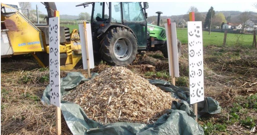
Wood volume within the compartment 2 was shredded, and shredded volume was measured with photogrammetry. The shredded volume was then converted to a solid wood volume using a conversion factor calibrated for the study on three batches of wood whose volume was known.
