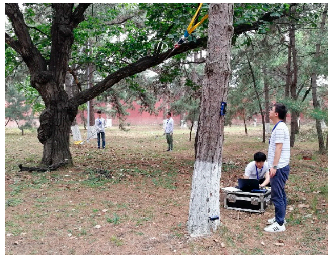
Figure 2. Field inspection of anchorage using the pulling test [45].
