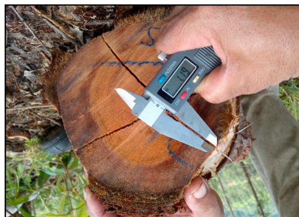
Figure 4. Measurement of split width for splits from pith to bark.
