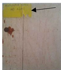
Figure 1. Acetylated birch plywood with an acetyl content of 30% from the 1945 research program was found in the FPL wood collection.
