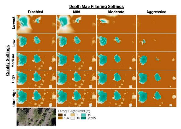
**Figure 3.** Subsets of filtered UAS-SfM point cloud-derived canopy height models (CHMs) (13 m  $\times$  30 m) for the 20 combinations of the build dense cloud Quality and depth map filter parameter settings. UAS-derived orthophoto of the subset area provided to aid in CHM inspection.
