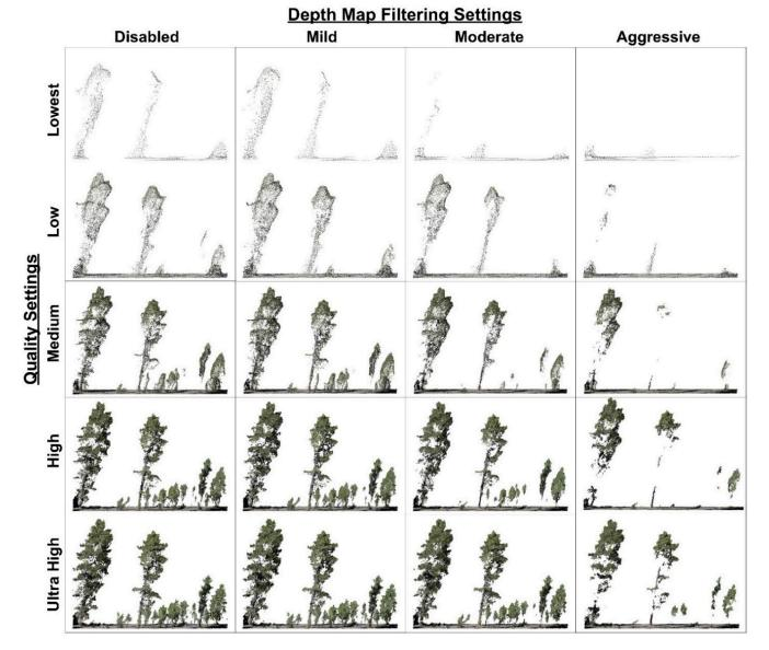
**Figure 2.** Subsets of filtered UAS-structures from motion (SfM) point clouds ( $15 \text{ m} \times 30 \text{ m}$ ) for the 20 combinations of the build dense cloud Quality and depth map filter parameter settings.
