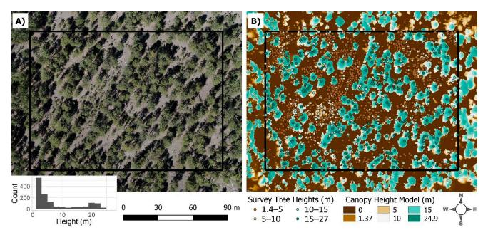
**Figure 1.** Study area portrayed with (**A**) unmanned aerial system (UAS) orthophoto at 2.6 cm resolution with inset distribution of survey tree heights and (**B**) UAS-derived Canopy Height Model at 10 cm resolution from High Quality and Mild depth map filtering with overlaid survey trees colored by height to demonstrate data alignment.
