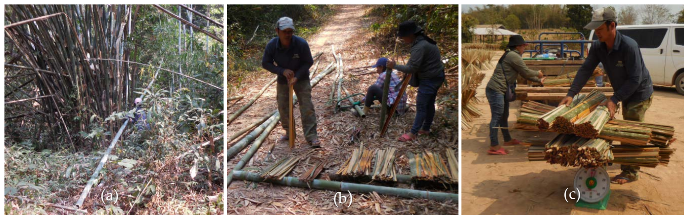
Figure 3. Bamboo harvesting and semi-processing steps: (a) villagers harvested whole bamboos in forest, (b) villagers cut and split bamboo stems (internodes) into smaller pieces on-site, and (c) villagers sold bamboo splits by weight to a company at the collecting area in town.
