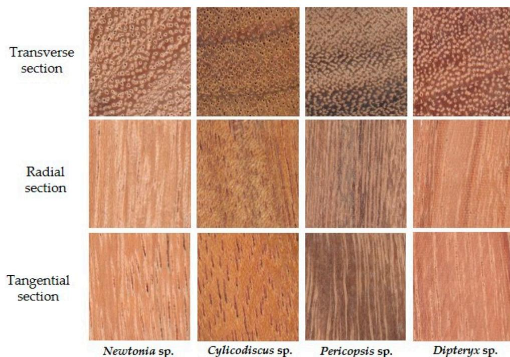
**Figure 2.** The three sections of the surface digital images from four timbers.
